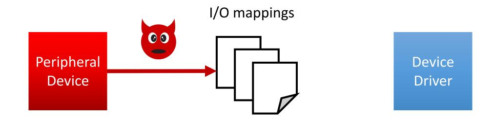
Attacker can write any value to the I/O mappings even multiple times at any time
